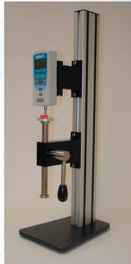
MT500L Lever-Actuated Tester with DFS Series force gauge, performing capsule crush test.
