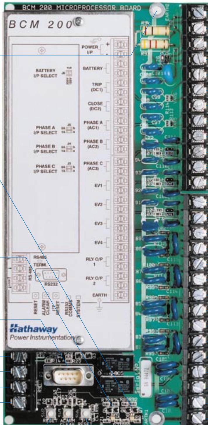
**Power Input** - ranging from 80 - 340Vdc, 85 - 264Vac.
