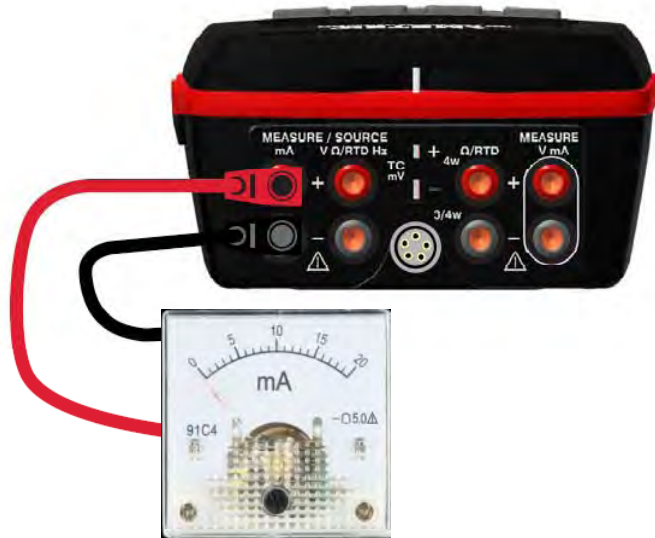
mA source Internal supply
