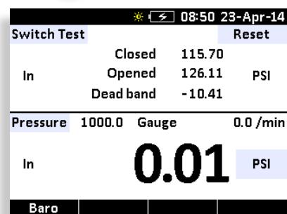
Automatic pressure switch test, records automatically, open, close and deadband values
