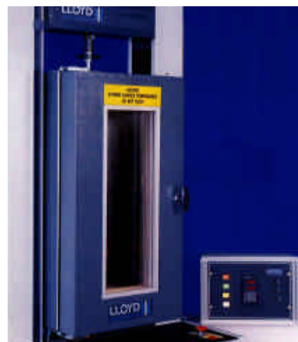
TC550 Cabinet with Temperature Control Unit
