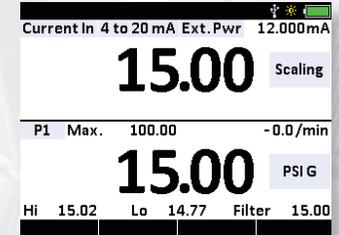
**% Error Calculation:** The HPC40 Series can calculate pressure vs. mA error as a percentage of the 4-20 mA loop span. For example, if you are testing a 30 psi full scale pressure transmitter with a corresponding 4-20 mA signal, you can program
