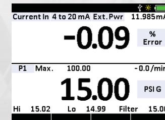
into the calibrator a 0 to 30 psi pressure span, and it will calculate and display the percent error in addition to the mA reading. This eliminates the need to manually calculate the error percentage. **Dampening:** If testing a pulsating pressure signal, use the dampening feature to smooth out the measurements, making them easier to read. **Min/Max:** With an update rate of 10 readings per second, the HPC40 Series is perfect for pressure safety valve testing.
