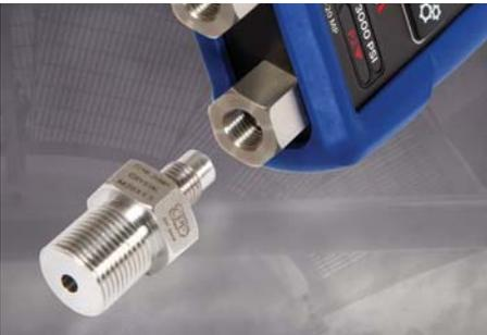
**CPF** Crystal Pressure Fittings♦ are machined in high-strength 316 Stainless Steel to operate at 10 000 psi/700 bar. Removable CPF adapters shift everyday thread wear away from the HPC40 Series' ports, while a self-venting weep hole alerts you before you disconnect from a pressurized system.
