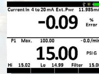
**Damping:** If testing a pulsating pressure signal, use the filter feature to smooth out the measurements, making them easier to read. **Min/Max:** With an update rate of 10 readings per second, the HPC50 Series is perfect for pressure safety valve testing.
