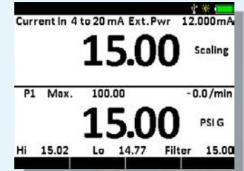
**% Error Calculation:** The HPC50 Series can calculate pressure vs. mA error as a percentage of the 4-20 mA loop span. For example, if you are testing a 30 psi full scale pressure transmitter with a corresponding 4-20 mA signal, you can program into the calibrator a 0 to 30 psi pressure span, and it will calculate and display the percent error in addition to the mA reading. This eliminates the need to manually calculate the error percentage.
