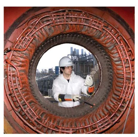
The Iris Power Corona Probe Model PPM-97 used to locate PD sites in a motor stator.
