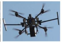
DayCor® Swift is a bi spectral UV-Visible camera with excellent scanning & corona detection capabilities, that fit monitoring of HV & MV electrical installations. Swift can be installed on a fixed mount or on a moving pan & tilt with 360° rotation or used on a UAS. Swift transmits during
